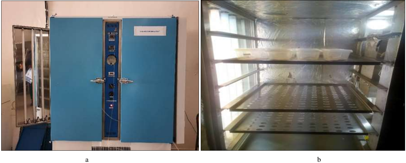
Fig 3: a) Climate Cabinet b) Containers in the climate cabinet at 5, 10, 15, 20 and 25 cm from the light.
